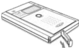
② Open the battery cover in the downward direction as the picture indicates.
