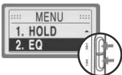
② Press the FF/REW button to move to EQ and then press the PLAY/STOP button to select.
