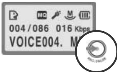
④ In the STOP state of ODE(or AUDIO MODE), press the REC button to start recording.
