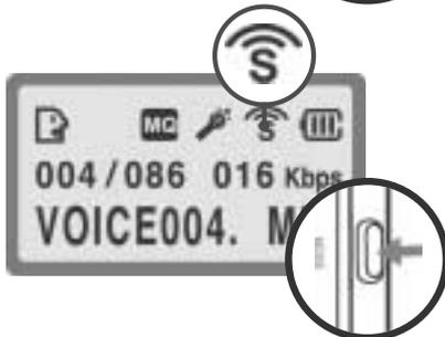
④ Press the MODE button to exit the menu. Make sure the icon on the LCD.
