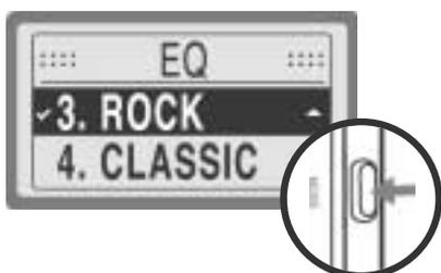
③ Press the FF/REW button to move to the desired equalizer mode and press the PLAY/STOP button to select. Press the MODE button to exit the MENU.
