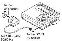
Plug the AC adaptor into the wall socket, and then insert the plug on the other end into the DC IN 3V socket.
