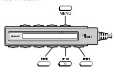
1 During playback or whilst in the stop mode, press the MENU button.
