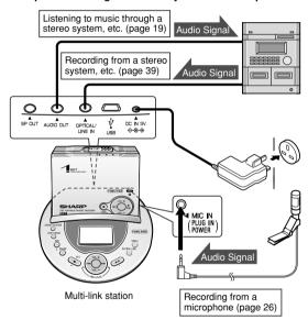
Note: SP OUT and AUDIO OUT sockets on the multi-link station accept 3-pole earphones, not the supplied 4-pole earphones.
