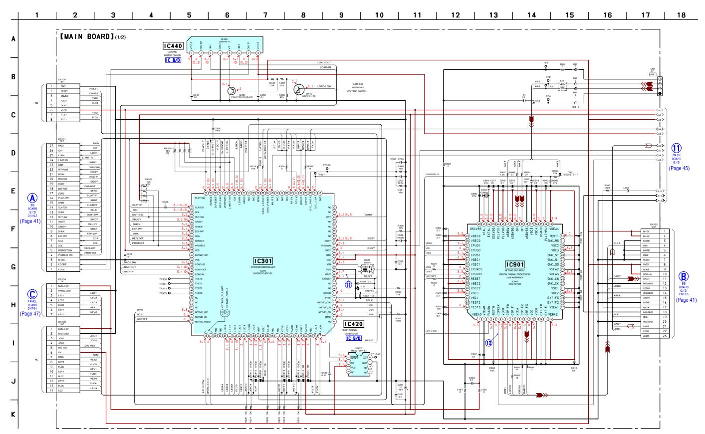
6-10. SCHEMATIC DIAGRAM – MAIN Board (2/2) – • See page 38 for Waveforms. • See page 48 for IC Block Diagrams.
