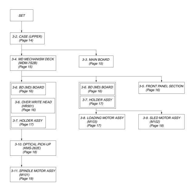
Note: Follow the disassembly procedure in the numerical order given.
