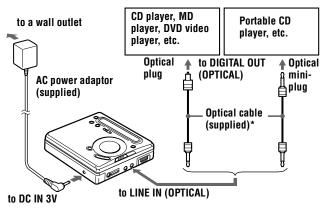
\* The supplied cable consists of one or the other of these cables. The shape of the plugs on the supplied cable may differ, depending on where the recorder was purchased.
