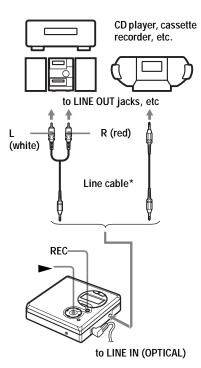
\* Use the connecting cords without an attenuator. To connect to a portable CD player having a stereo mini-jack, use a connecting cord with a stereo-mini plug on both ends (not supplied).
