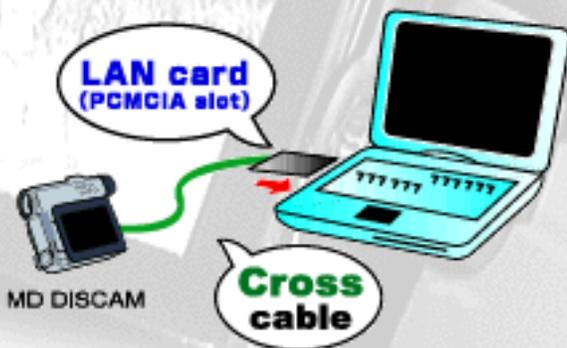
If you have a laptop, insert a LAN card in the slot of your PC. Refer to the instruction manual of the LAN card about its installation.
