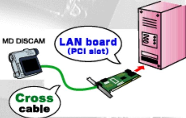
A commercially available LAN board or LAN card is required to add an Ethernet Terminal to the PC.
